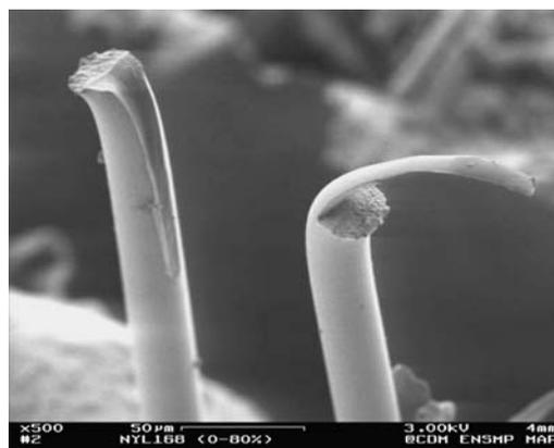
Figure 3 Typical fatigue fracture morphology of a PA 66 fiber.
